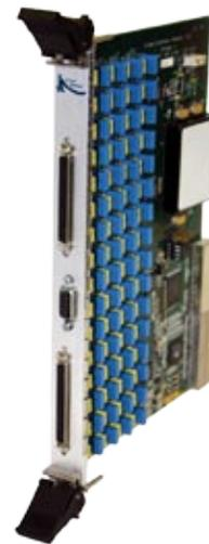
KineticSystems' CP266 is a single-width, 6U, CompactPCI module with 32 or 64, 16-bit analog output channels
