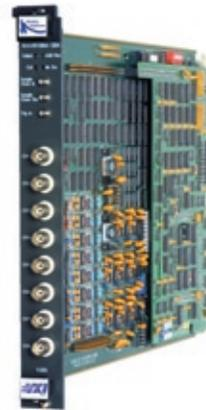
A high-resolution multichannel arbitrary waveform generator
